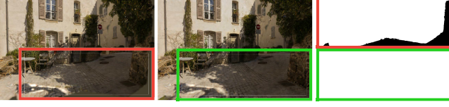
Figure 2: With a limited budget of cameras, i.e., N = 4 , we see the importance of camera selection even in simple scenes like Ponche. Left is the camera selection method of [RK20]. In the middle is ours and on the right we show a mask with black for missing content. In the top right (red), we see that the first method clearly fails to provide information for the whole frame, while ours (bottom, green) with the same number of cameras covers the frame.
