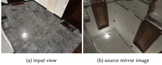
Fig. 5. For in each input view (a), we compute a mirror image (b) by tracing a ray in the mirror direction of the first mesh intersection and sampling the image whose camera–intersection vector makes the smallest angle with the mirror direction (see also Figure 6). Mirror images help the network analyze scene materials, and identify complex glossy effects like the salient highlight on the floor.
