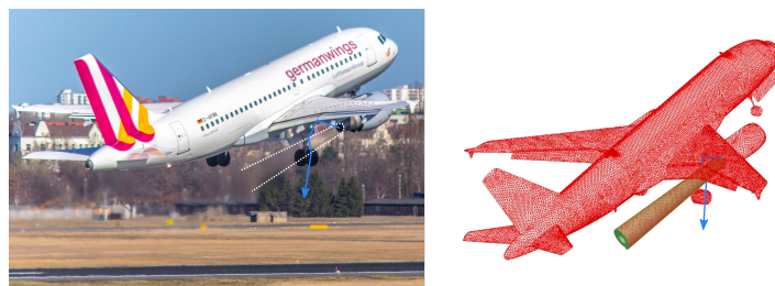
FIGURE 1 – An acoustic wave (blue arrow) emitted by the aircraft's engine, reflected on the wing and crossing the jet of exhaust gas. Real-life case (left) [22] and a numerical model example (right). The red 2D mesh represents the aircraft's surface and the surface of the green 3D cylinder volume mesh representing the exhaust flow.
