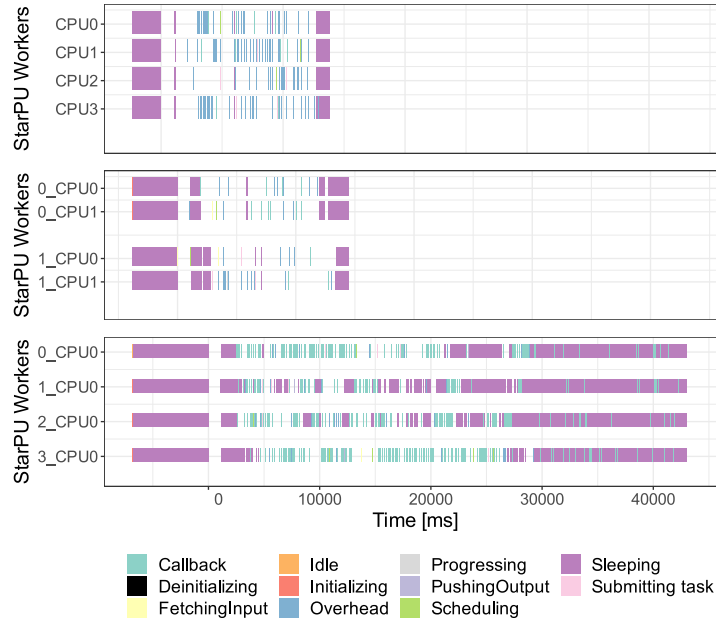
FIGURE 23: Graphical visualization of the execution traces provided by the StarPU runtime corresponding to the execution of HMAT on a BEM system having 25,000 unknowns using 1 MPI process times 4 StarPU workers, 2 MPI processes times 2 StarPU workers, 4 MPI processes with 1 StarPU worker per process on a single miriel node respectively. Blank spaces represent the time spent in computation. The colors represent the actions of the StarPU runtime. Out-of-core has been disabled.
