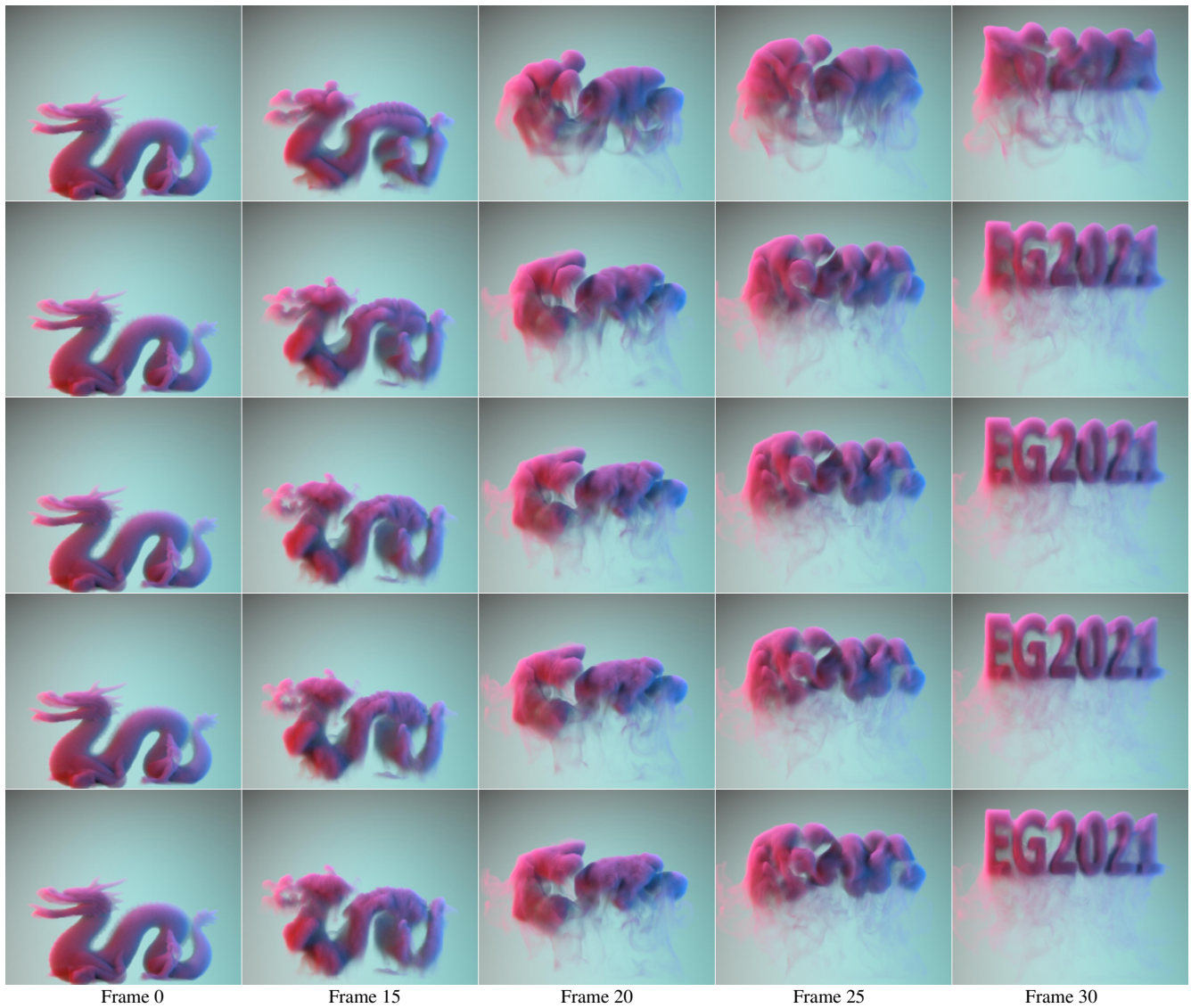
Figure 13: 3D dragon example resolution 200 \times 170 \times 60 . The density is first initialized with a dragon-shaped volume, and the letters of EG2021 are specified as target. Our optimization results at different frequency bands are shown. From the top to the bottom, the cutoff wavenumber k_c is 1, 3, 8, 23, 64 respectively.
