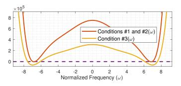
Fig. 2. The evaluation of  $C_1(j\omega)$  and  $C_2(j\omega)$  of eq. (4) and of  $C_3(j\omega)$  of eq. (7) of a non-passive transfer function, observed by  $C_3(j\omega)$  being negative at some real values of  $\omega$ .
