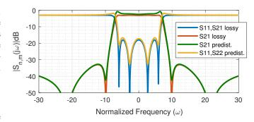
Fig. 1. Lossy scattering parameters obtained by scaling by 3dB a Cauer (elliptic) 4th degree function (blue and red traces) and predistorted version with  $\sigma=-0.25$  (green and orange traces). The predistorted version is the one considered for the example of section III-B
