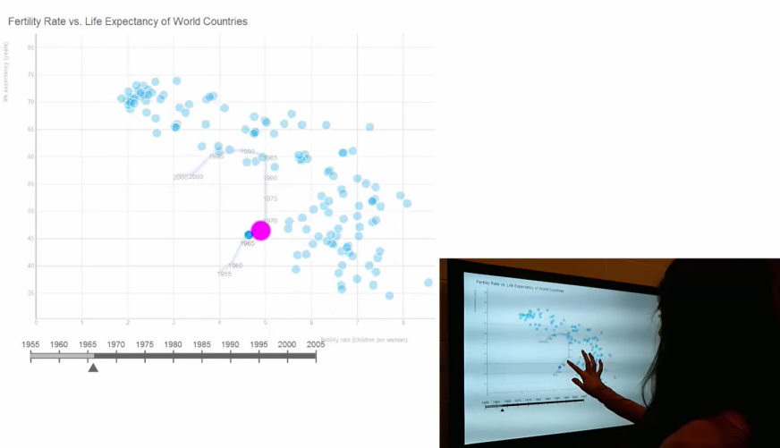
Figure 2.6: With DimpVis (Kondo and Collins, 2014), users can select a data item and follow visual hint paths that indicate how the selected item has changed over time using touch. (The visual hint path is shown as a gray line while the pink and blue dots indicate a finger point and currently selected item, respectively.)
