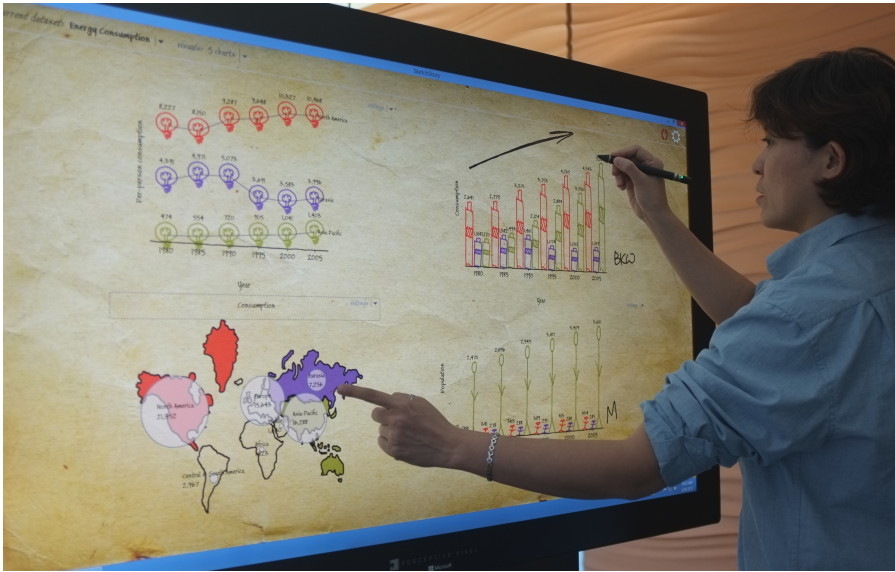
(a) SketchStory recognizes a few sketch gestures for chart invocation, and automatically completes charts on the fly using presenter-provided icons and binding them to the underlying data.
