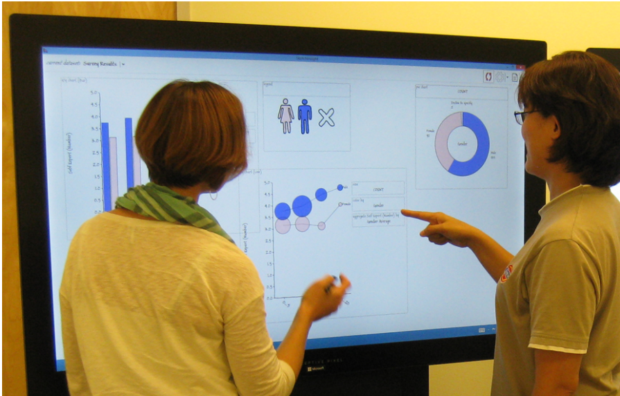
(b) SketchInsight allows people to visually explore the data by drawing simple charts and directly manipulating them with pen and touch interaction.
