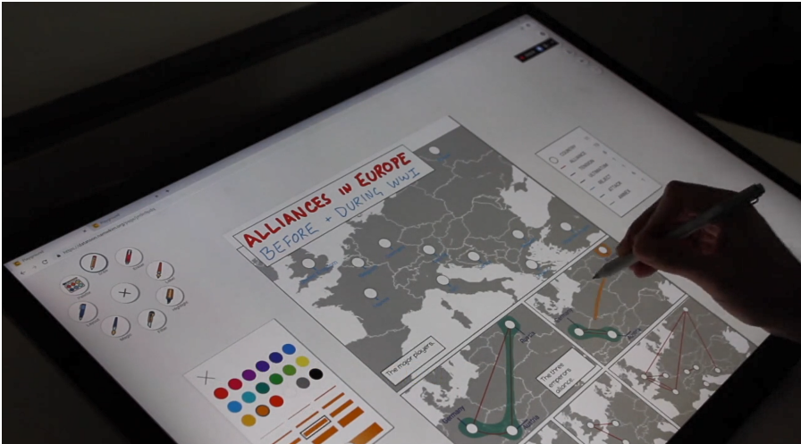
Figure 2.7: DataToon (Kim et al. , 2019a) is a storyboarding tool that facilitates the creation of data comics focusing on network data by blending analysis and presentation in a unified environment supported by pen and touch interactions.
