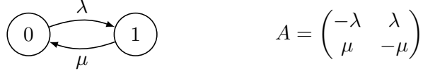
FIGURE 7. The two-state irreducible continuous time Markov chain X , where \lambda > 0 and \mu > 0 .
