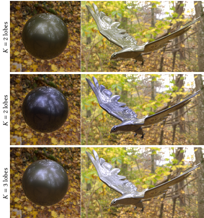
Fig. 22. Stacking up to 3 lobes. The top two rows show materials made of two lobes: a smooth 1-layer dielectric coating ( R_1 = 0.03 ) onto either of two rough dielectrics: a yellowish 2-layer lobe (top, \mathbf{R}_Y = [0.1, 0.1, 0.06] , \sigma_Y = 0.05 ) or a blueish 1-layer lobe (middle, \mathbf{R}_B = [0.05, 0.05, 0.09] , \sigma_B = 0.01 ). The last row uses all three lobes, with the yellowish lobe at the base and the blueish lobe in the middle.
