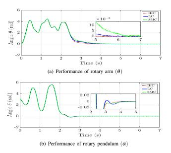
Fig. 3. Comparison of the performance in the IP stabilization
