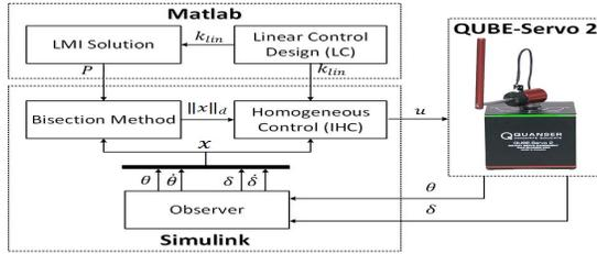
Fig. 2. QUBE<sup>TM</sup> Servo 2 in closed-loop with the IHC.
