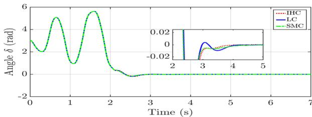
(b) Performance of rotary pendulum ( $\alpha$ )
