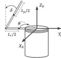
Fig. 1. Schematic diagram of inverted pendulum (IP)
