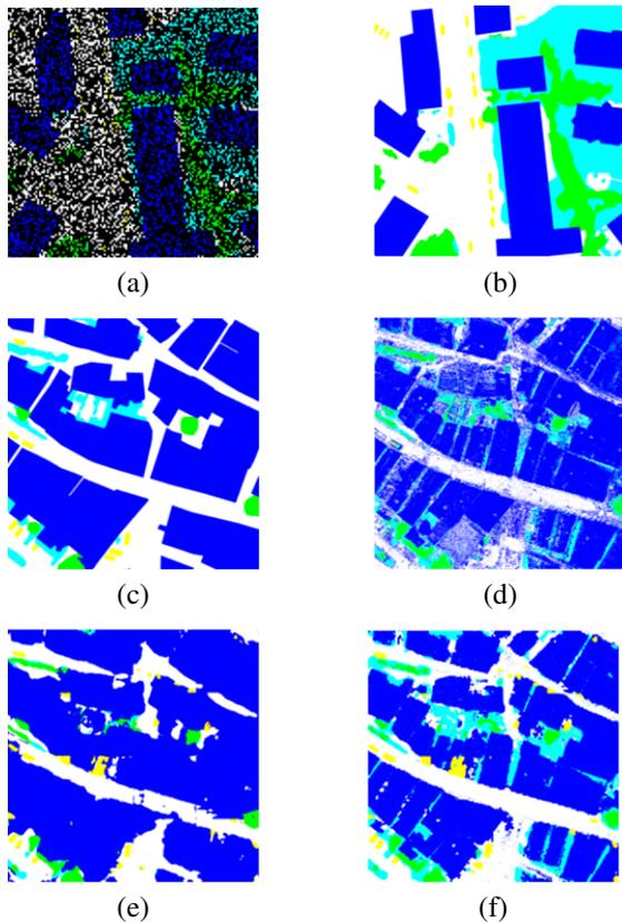
**Fig. 1. Ground truth and classification maps:** (a) training set with 70% of unlabeled pixels, (b) original training set, (c) test set; classification maps: (d) RF, (e) U-Net, and (f) the proposed method (“resize”). Classes: buildings (blue), impervious (white), vegetation (cyan), trees (green), cars (yellow).
