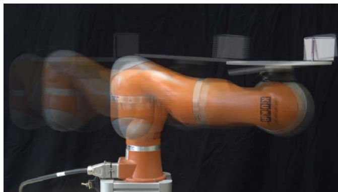
Fig. 1. A teleoperated 7-DoF robot manipulator transports an object in a nonprehensile configuration while autonomously modulating the user-specified inputs and the object orientation to prevent it from sliding and possibly falling under the action of gravity.
