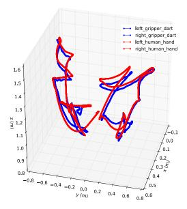
Fig. 3. Grippers and human hands trajectories during teleoperation The human hand trajectories are representated in red and are given as a reference to the whole-body control framework. The simulation is run thanks to robot\_dart. Talos' grippers trajectory in the simulator are represented in blue. The tasks, contacts and constraints used are in Table I.
