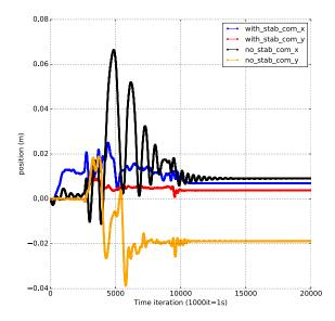
Fig. 2. **COM planar xy trajectory during a double support teleoperation test** Teleoperation references are given to a simulated Talos in robot\_dart (Fig. 3). The references are given twice faster than in Fig. 4 and Fig. 5 which leads to COM instability. The blue and red plots are the output trajectory with our activated stabilizer. The black and orange plots are without stabilization.
