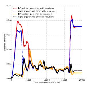
Fig. 4. **Grippers Position error during teleoperation** This corresponds to the Fig. 3 trajectory. At the beginning and end of the teleoperation experiment, the human hands are overlaid to Talos hips and the repulsors prevent any collision.
