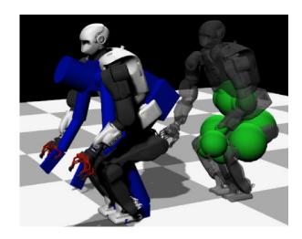
Fig. 1. **Talos teleoperation behavior simulated in robot\_dart.** The 66 degrees of freedom human model is displayed as a graphical object in blue. It is overlaid to the simulated Talos. The grey Talos is also a pure graphical object (no forces, gravity, physics...) showing the direct whole-body control output solution. The green spheres are the display of the repulsors of the left gripper.
