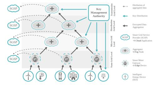
**Fig. 2.** The lowest layer includes the consumers and generators. In the higher layers, only aggregators reside. Aggregators can not decrypt the aggregated values. Possible data flow is indicated by the arrows. Only the Smart Grid Service Providers have access to the aggregated data. Authorization is based on the aggregation level.
