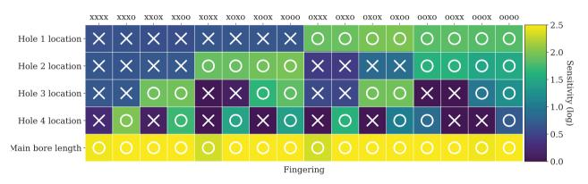
Figure 5. Sensitivity of the reflection coefficient w.r.t the hole locations/bore length design parameters (Eq. (34)) for frequencies in [0.1, 4] kHz with a 2 Hz step. Open (resp. closed) holes are indicated with circles (resp. crosses).
