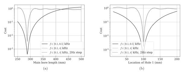
Figure 6. Cost evolution along one dimension of the design space for three frequency ranges: [0.1, 0.5] kHz and [0.1, 4] kHz with a 100 Hz step, and [0.1, 4] kHz with a 2 Hz step. (a) Total length  $L_{mb}$ , fingering: xxxx". (b): Location of hole 1  $X_{h1}$ , fingering "oxxx".
