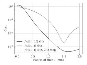
**Figure 7.** Cost evolution with respect to the radius of Hole 1 on the fingering "oxxx", with three frequency ranges: [0.1, 0.5] kHz and [0.1, 4] kHz with a 100 Hz step, and [0.1, 4] kHz with a 2 Hz step.
