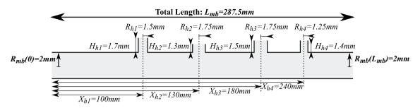
Figure 1. Sketch of the cylindrical tube with four side holes to be recovered. It is described by 15 geometric parameters (three for the main bore profile and three for each of the four holes).
