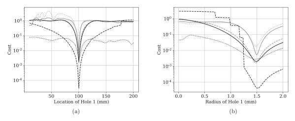
**Figure 4.** Costs evolution for different observables computed for frequencies in [0.1, 4] kHz with a 2 Hz step, for the fingering "oxxx" with respect to: (a) the location and, (b) the radius of the first hole. The observables are: the complex value (solid lines), the modulus (dotted lines) and the phase (dashed lines) of the impedance (gray) and the reflection coefficient (black).
