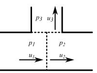
Figure 3. Sketch of a T-junction with the adopted convention for the flow orientation.
