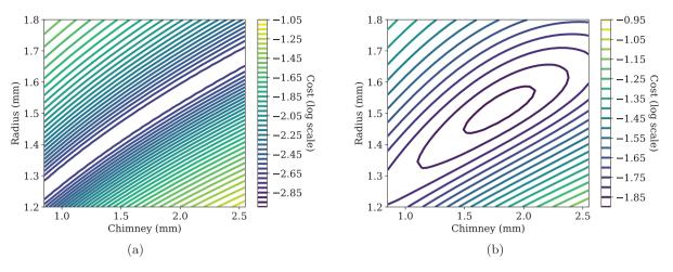
Figure 8. Cost corresponding to the reflection coefficient, with respect to the first hole radius  $R_{h1}$  and chimney height  $H_{h1}$ , for frequencies in [0.1, 4] kHz with a 0.1 kHz step. (a) The fingering for which only the first hole is open (oxxx). (b) Five fingerings (xxxx, xxxo, xxxx, xxxx, xxxx)
