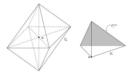
Figure 8: Interior vertex patch (left) and the element  $K_1$  with the face  $F_1^{\text{ext}}$  (right)
