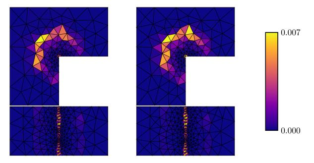
Figure 7: [Singular solution (6.3)] Estimated (left) and actual (right) error distributions at adaptive mesh refinement iteration #10. Top view (top) and side view (bottom).
