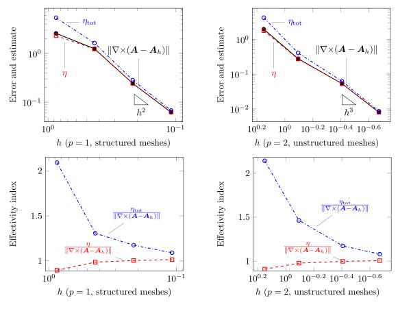
Figure 3: [Analytical solution (6.2)] Uniform mesh refinement.
