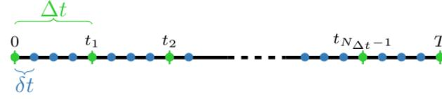
**Figure 1:** Definition of the temporal discretization of the fine and the coarse propagators (respectively bullets and vertical traces). The instants  $t_n, n = 0, \dots, N_{\Delta t}$  correspond to the coarse discretization.
