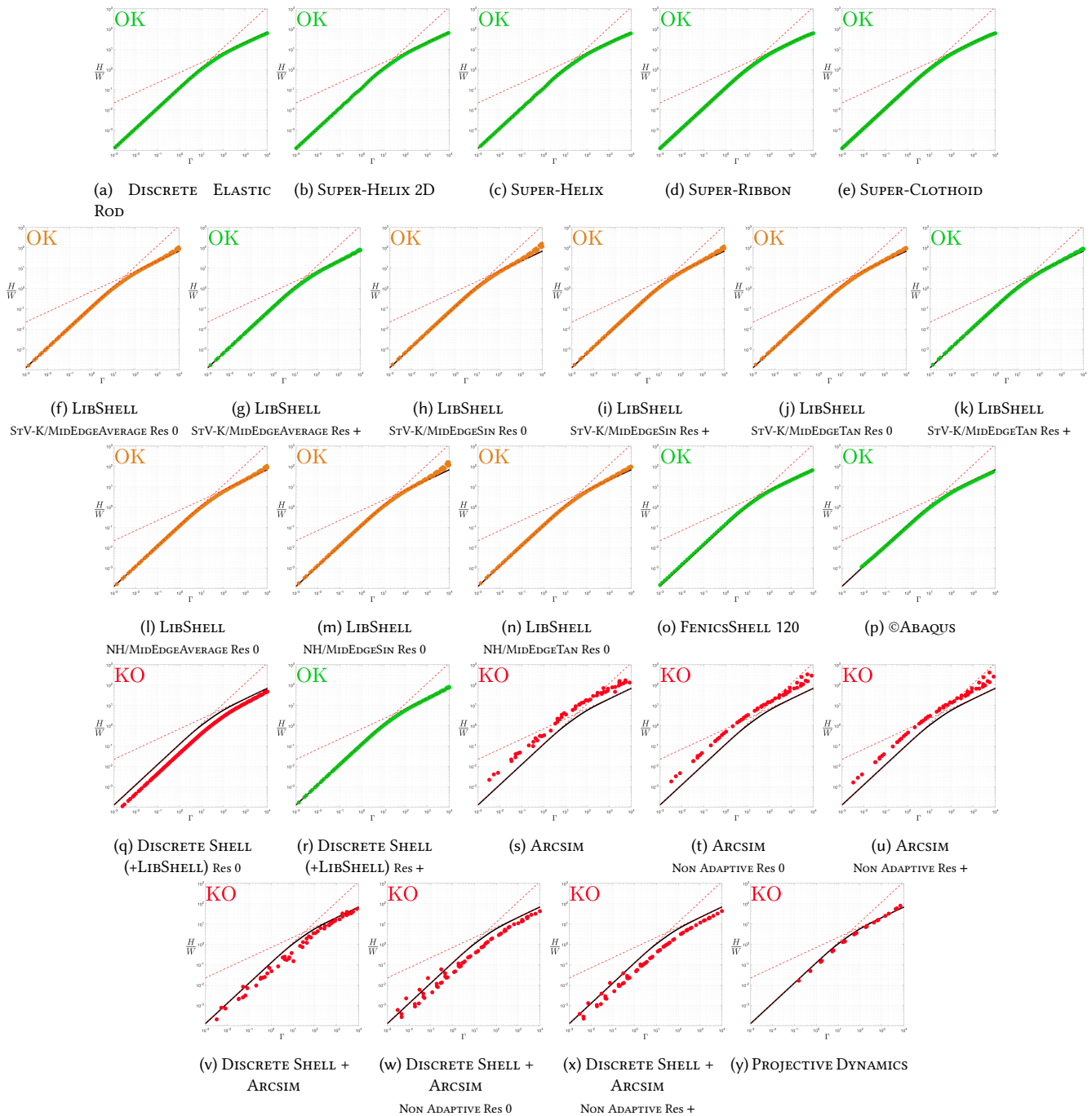
Fig. 27. Full results on the Cantilever test. NH stands for Neo-Hookean.
