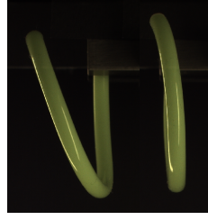
Fig. 22. Bend-Twist transition. (Left) 3D rod, with L = 9.6 cm. (Right) 2D rod, with L = 9 cm.
