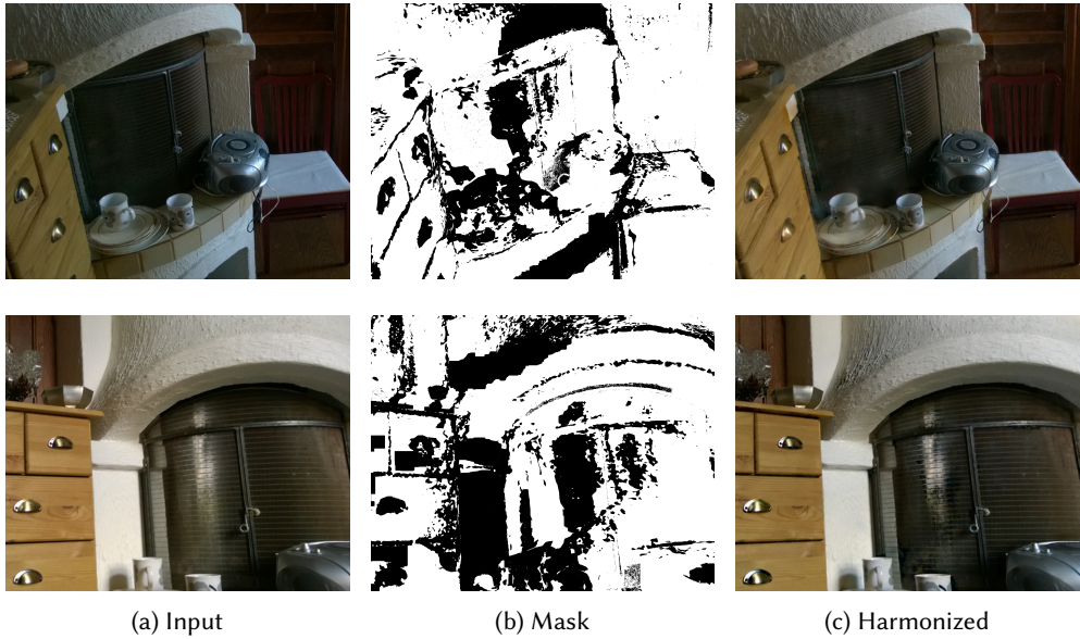
Fig. 6. Harmonization: From an input image (a) exhibiting significant appearance variation, we obtain harmonized images (c). A mask (b) alleviates specularly suppression.
