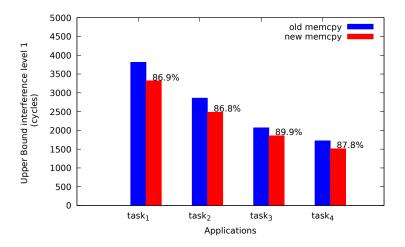
Figure 4: L1 interference reduction after memcpy optimization
