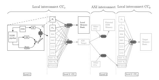
Figure 2: Memory system of the MPPA3 processor
