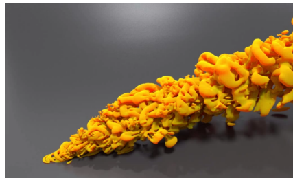
Jet in crossflow (Q-isosurfaces)
