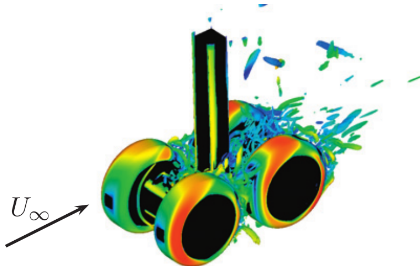
PANS simulation of the flow around a rudimentary landing gear (Q-isosurfaces colored by the velocity magnitude)
