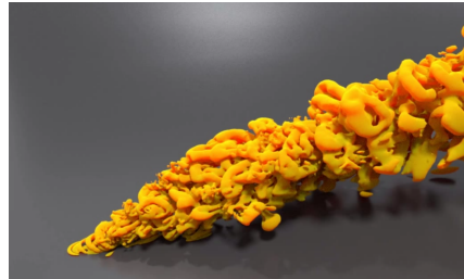
Jet in crossflow (Q-isosurfaces)
