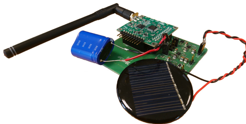
Figure 3. Single-task IoT node platform.
