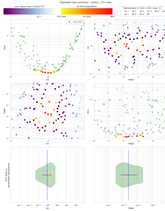
Fig. 3. Restricted search on the IS parameter, for the Lorenz task. With a value of 1, we can see that the IS yields the best results and reaches the minimum of the U-shaped error cloud that can be seen in the top-left plot.
