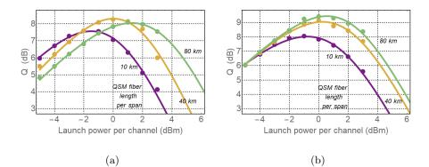
Fig. 2: Q-factor as a function of the total launch power per channel. (a) No MPI compensation; (b) 100% MPI compensation. (Symbols: Points: Monte Carlo simulations; Lines: Least squares fitting using (1) with  $\tilde{a}, \tilde{\beta}, \tilde{\gamma}$  as unknown parameters.)
