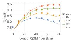
Fig. 3: Optimum Q-factor  $Q_0$  as a function of the QSM fiber length  $\ell_{s_1}$  per span. (Symbols: Points: Monte Carlo simulations; Lines: Least squares fitting using (1)-(4) with  $\epsilon$  as an unknown parameter. Here  $\epsilon \simeq 0.2$ .)
