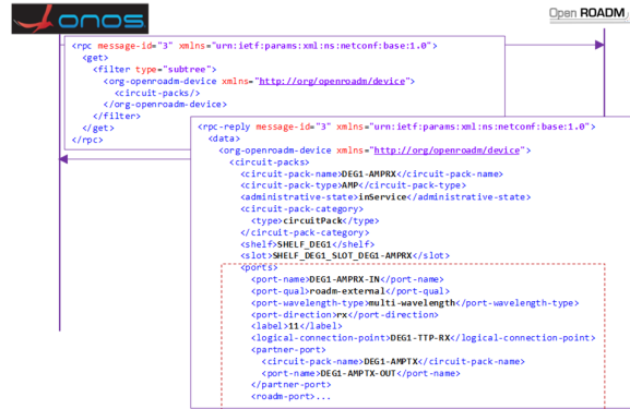
Fig. 8. NETCONF <get> operation to retrieve the list of circuit packs of the OpenROADM.
