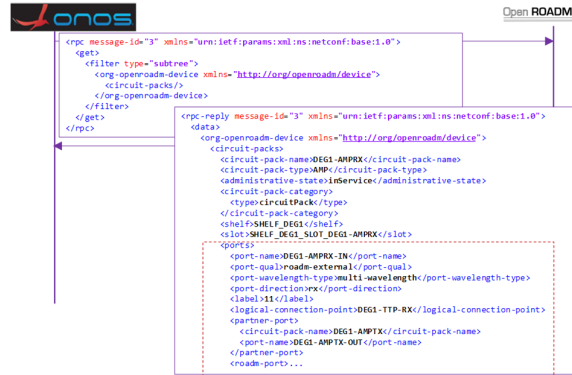
Fig. 8. NETCONF <get> operation to retrieve the list of circuit packs of the OpenROADM.
