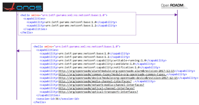
Fig. 7. Initial Capability Discovery between the SDN controller and the OpenROADM.
