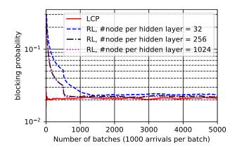
Fig. 3. Performance of RL-routing with LCP fitting.
