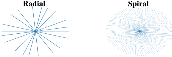
Fig. 2. Schematic representation of the two multi-shot non-Cartesian (radial and spiral) readouts considered here for 2D imaging. In our setting, we used N_s = 100 shots, each of them consisting of 640 samples giving a total of m = 64,000 k-space measurements. Here only 9 shots are presented.
