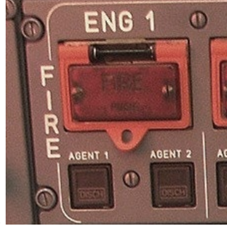
Fig. 4. Engine 1 FIRE push-button on the overhead panel.
