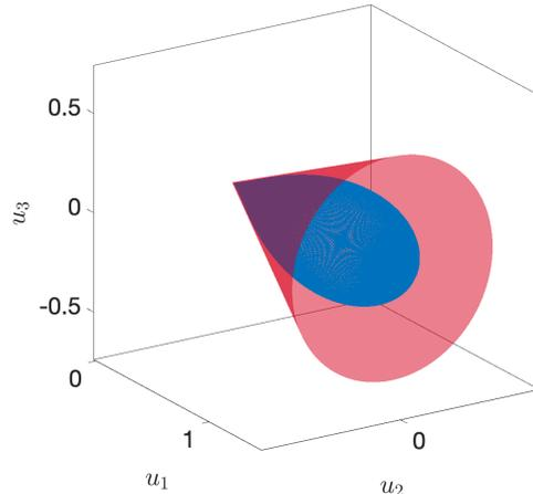
Fig. 1. Example of orbital control with solar sails. Equations are of the form of System (1), the control  $u = (u_1, u_2, u_3)$  is homogeneous to a force, and the solar sail only allows forces contained in the set  $U$  figured in blue in the picture (for some characteristics of the sail). The minimal convex cone containing the control set  $U$  is depicted in red. Neither  $U$  nor this cone are neighborhoods of the origin.
