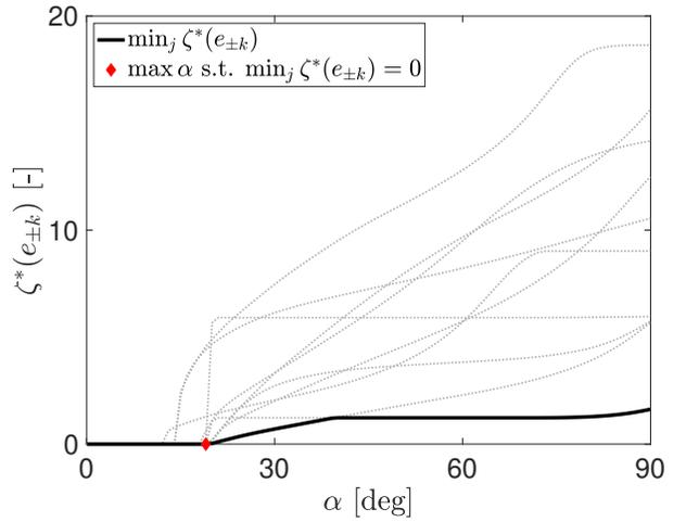
Fig. 6. Grey lines show the resulting displacement  $\zeta^*$  toward all positive and negative base vectors, i.e.,  $e_{\pm k} = \pm \partial / \partial I_k$ ,  $k = 1, \dots, n$ . Black line shows the minimum of these curves. The minimal angle  $\alpha$  ensuring local controllability is highlighted in red. One can notice that some curves do not strictly increase, but are constant instead. It means that the control is inside the cone, and increasing  $\alpha$  does not change the result.
