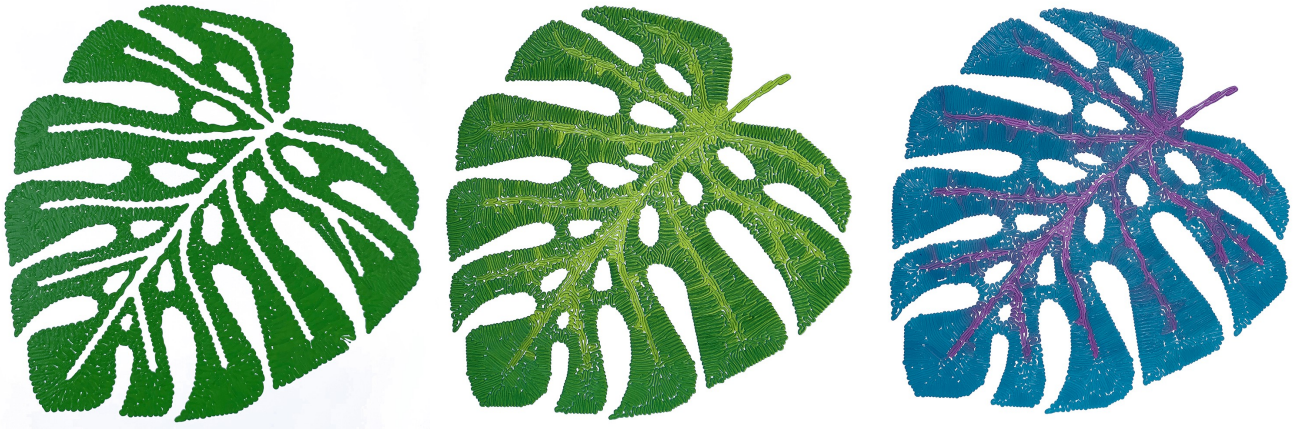
Fig. 20. Left: Single material leaf printed with a constant width smaller than nominal to appreciate the cycle folds. Note how the cycle goes around holes with a single folded trajectory in the center part. Middle: Multi-material version using a narrower spacing, with the inner skeleton in a different material. Right: Variant using different colors.
