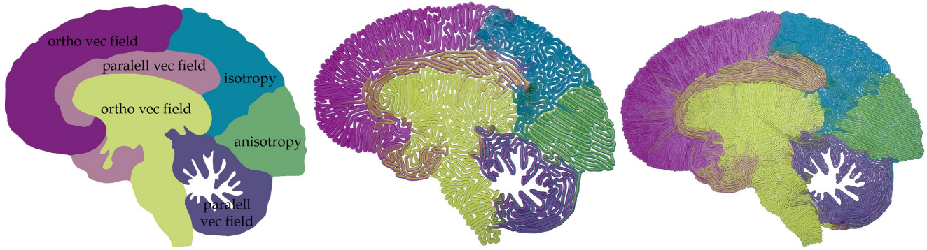
Fig. 19. Left: input specifying zones and objective selection in each. Parallel vec field means that we align the path with a vector field parallel to the zone border and ortho vec field means that we use alignment with a vector field orthogonal to the border. Middle: cycle optimized for a width of 1.7mm. Right: cycle optimized for a width of 0.8mm.
