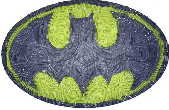
Fig. 17. Multi-material printing of the Batman logo following the parallel vector field.
