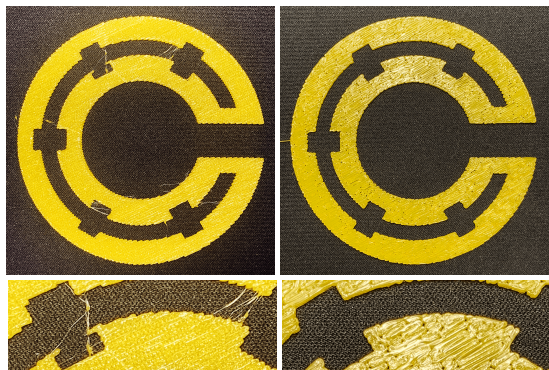
Figure 24: Comparing a standard zigzag strategy and our anisotropic infill. Left: While the zigzag is perfectly regular, it does not allow for continuous extrusion. Travel moves create marks and oozing, that damage the final part. Right: None of these issues are present on our fully continuous 3D prints.
