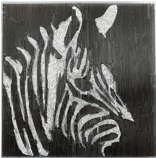
Figure 20: Zebra printed with black and white filaments.
