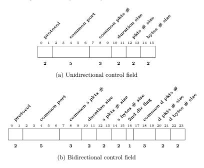
Fig. 3. CompactFlow control fields (in bits).
