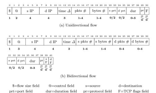
Fig. 2. Binary schema of CompactFlow records (in bytes).
