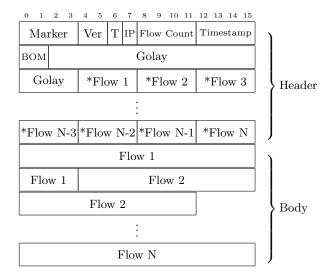
Fig. 1. CompactFlow file format (in bytes).
