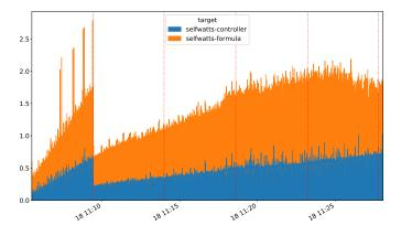
Fig. 9. DRAM power consumption of the  $\ensuremath{\mathsf{Controller}}\xspace/\ensuremath{\mathsf{Sensor}}\xspace$  and Formula components
