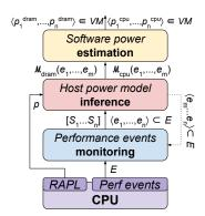
Fig. 1. Overview of the SELFWATTS approach.
