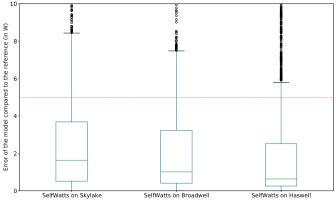
Fig. 10. Estimation errors  $\varepsilon$  for SELFWATTS on across different CPUs
