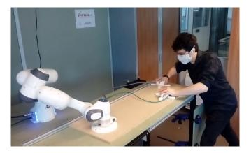
Fig. 1. Subject performing an experiment of a milling task in carpentry using a physically realistic mock-up. The wooden part is being pushed through handles incorporating 6-axis F/T sensors. A 7-DOF collaborative robot is attached to the wooden part and reproduces the cutting forces based on a wood cutting model [9].
