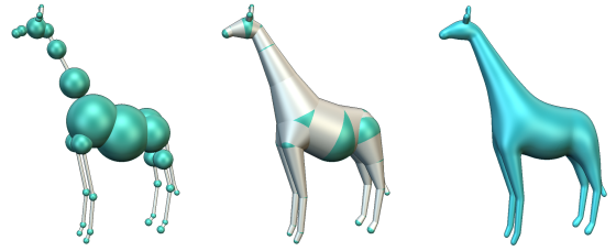
Figure 2: Left: a skeleton with prescribed radius on its vertices, Middle: infinite union of spheres defined by linear interpolation of prescribed radius along skeleton edges (this is also a union of sphere-cone), Right: resulting scale-invariant integral surface which can be seen as a smoothing of the sphere-cone union.
