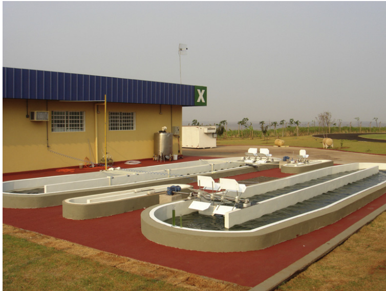
FIGURE 1.4 Pilot plant for microalga cultivation using vinasse and carbon dioxide in the medium.
