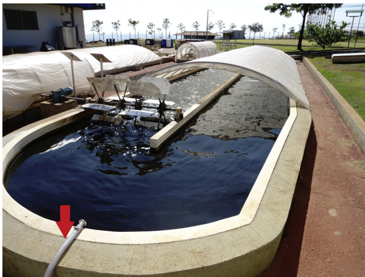
FIGURE 7.4 Open ponds for microalgae cultivation at Ourofino Agronegócio, Brazil.
