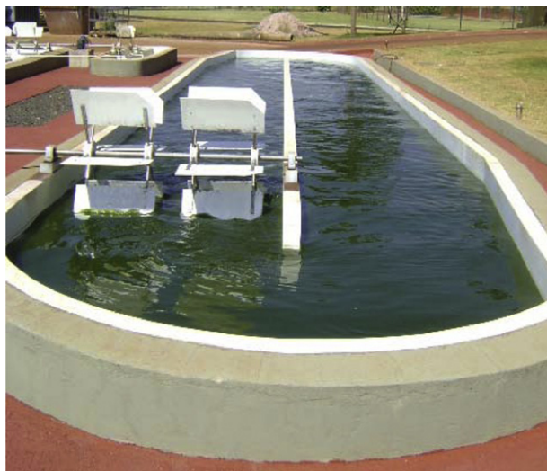
FIGURE 4.4 Paddlewheel mixing of raceway ponds at Ouro Fino Agronegócio (Brazil).
