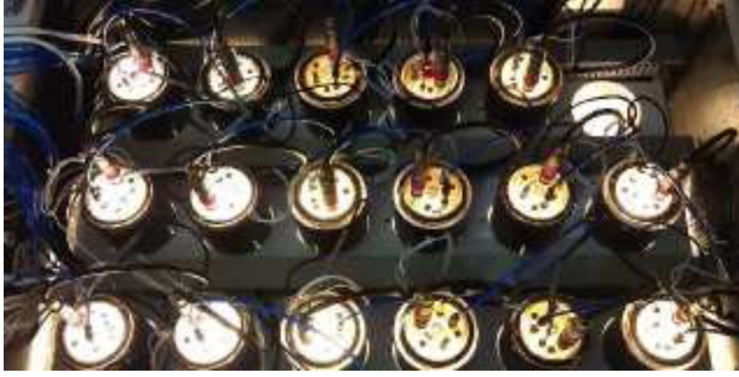
Fig. 1. The TIP system. The device has 18 batch photobioreactors for microalgae cultivation.
