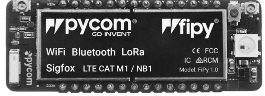
Fig. 2 – FiPy board from Pycom [18].
