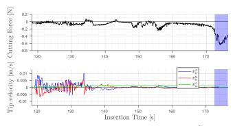
Fig. 7. Cutting force  $f_t^z$  and tip insertion velocities  $\mathbf{v}_n = [v_n^x, v_n^y, v_n^z]$  in a representative insertion in modality  $G_K C_V$ . The blue-shaded area represents the time when the armband was vibrating.
