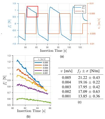
Fig. 4. Friction force estimation. (a) Time vs. force applied on the needle  $f_s^z$  (blue) while applying alternated step velocities  $v_i=\pm 0.005$  m/s (orange) along the needle axis direction. (b) Time vs. force applied on the needle for different velocity magnitudes  $v_i\in \mathbf{v}$  during needle extraction (magnification of the red square sector above). (c) Friction per unit length  $f_f$  for different insertion velocities v.
