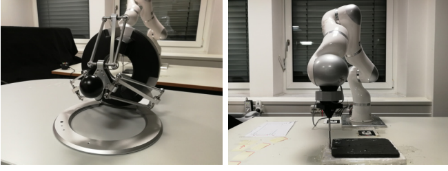
Fig. 2. Experimental setup used for validating our approach on a cutting task. Left: Our Omega3 haptic device used as master. Right: Our 7 DOF KUKA lightweight robot with a mounted cutting scalpel. The black clay is placed on a piece of foam on the table and serves as the material to cut.
