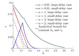
Fig. 3. Bounds on  $\bar{h}$  and  $\bar{\tau}$  for the LTI system (44) in the large-delay case (in red), and in the small-delay case (in blue), for  $\alpha = 0.01$  (solid line),  $\alpha = 1$  (dashed line) and  $\alpha = 2$  (dotted line). The analytical stability bounds on constant  $h_k$  and  $\tau_k$  are given by the green line [35].
