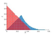
Fig. 1. Feasible values of  $\bar{h}$  and  $\bar{\tau}$  for the nonlinear system (37) with  $\alpha = 0.1$ , in the large-delay case (in red), and in the small-delay case (in blue).
