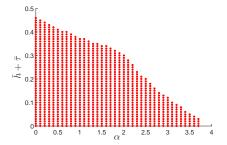
Fig. 2. Trade-off between desired decay-rate  $\alpha$  and  $\bar{h} + \bar{\tau}$  for the nonlinear system (37), in the large-delay case.
