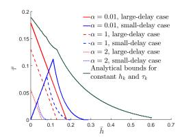
Fig. 3. Bounds on h and  $\bar{\tau}$  for the LTI system (44) in the large-delay case (in red), and in the small-delay case (in blue), for  $\alpha = 0.01$  (solid line),  $\alpha = 1$  (dashed line) and  $\alpha = 2$  (dotted line). The analytical stability bounds on constant  $h_k$  and  $\tau_k$  are given by the green line [35].
