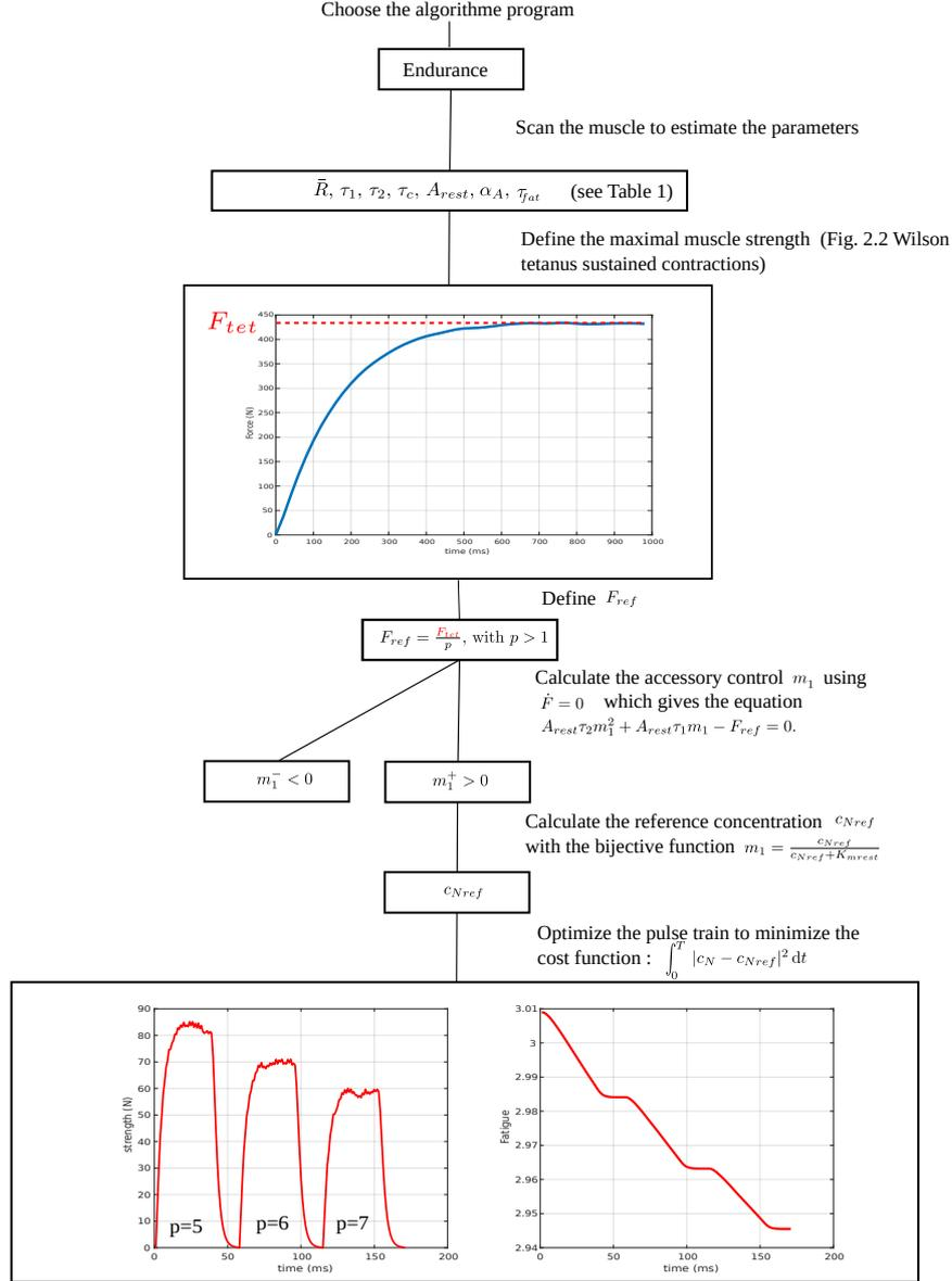
Fig. 6. Endurance program for a smart electrostimulator.
